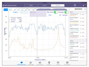
Spectral view shows interference within a channel
