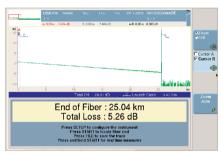
Figure 2 Fault locator mode
