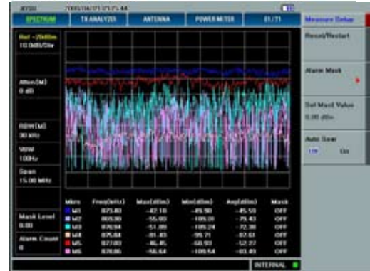
Fig 8 – RSSI view for intermittent signals
